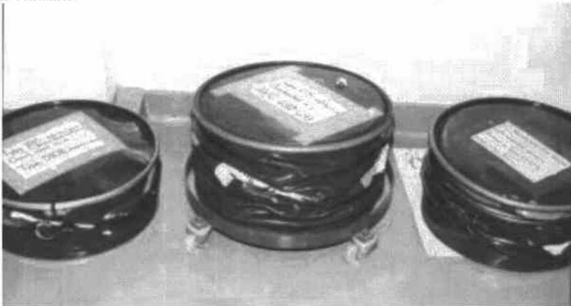
Figure 1. AMWTP pucks produced by supercompaction of 55-gallon drums of debris waste.
