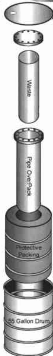
Figure 4. Photograph of a 12-inch-diameter pipe overpack and schematic diagram of the loading scheme for a 6-inch-diameter pipe overpack.
